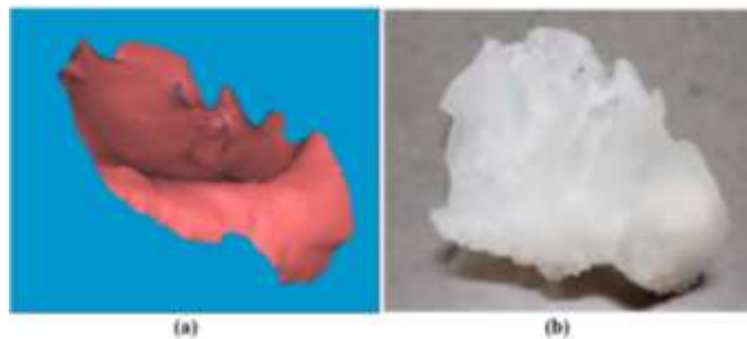
(a). Implant 3D CAD model (b). 3D printed implant
