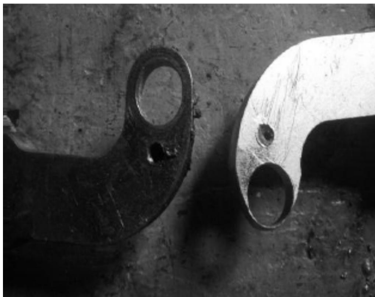
Figure 10. Bracket Fixture Comparison after and before Milling and Plating
