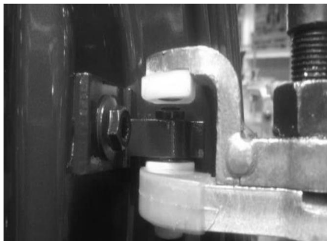
Figure 8. Increased Gap between Door and Locking Nut
