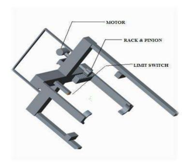
Fig.1 CAD model of recue robot
